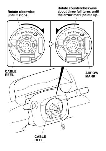
21. Route the airbag connector through the opening in the new steering wheel, then install the steering wheel to the steering column shaft in the straight-ahead position: Make sure the wire harnesses are not pinched.
