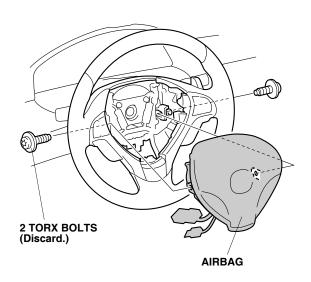
7. Unplug the vehicle connector from the cable reel, and loosen the steering wheel bolt.
